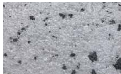
EXPOL StyroDrain is made from 100% Recycled Polystyrene
